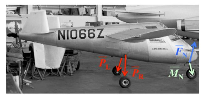
In this problem, you should imagine that you're Ed Lesher and are sizing the landing gear for <u>actual operations</u>. In other words, you should try to think about the <u>operational scenario</u> that puts the greatest load on the landing gear (e.g. *not* sitting unused in the FXB atrium, in flight, etc.).
